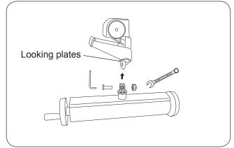
**Liko MasterLift, Likorall (not R2R) and Golvo** FlexoStretch is assembled using M10x25 screws and nuts directly into the lift's looking plates. Recommended tools: 6 mm Allen wrench and 17 mm closed-end wrench.
