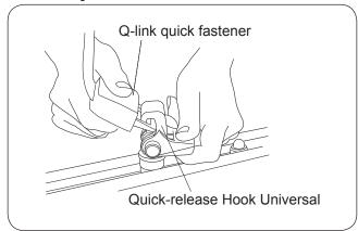
Assembly with Quick-release Hook
